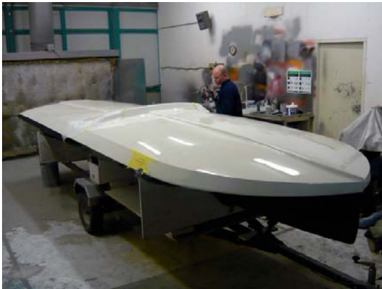
(a) The PV sportsboat spray-painted.
