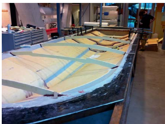
(c) Supports for the deck of the Liyang-boat.
