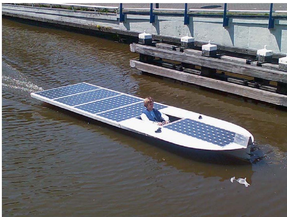
Figure 8.2: PV boat of 6 m long and 1.5 m wide with five conventional 175 Wp glass-based PV modules placed on its deck (picture taken by author).
