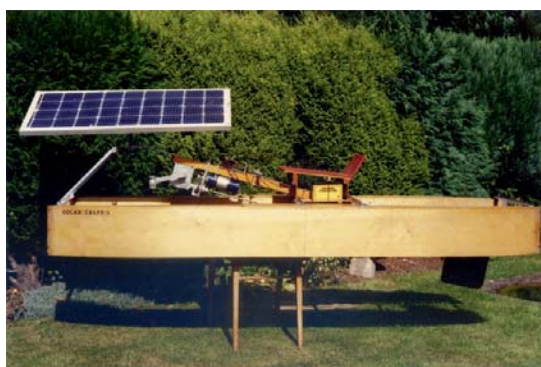
Figure 1.6: Solar Craft 1. A PV-powered boat built in 1975 by Alan Freeman [28].
